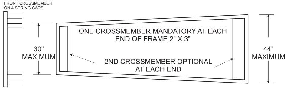
ENTIRE FRAME MUST BE 2" X 3" X .100" MIN. WALL THICKNESS
